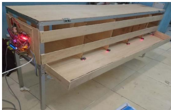
Gambar 3. Kandang Ayam Terintegrasi Sensor Tampak Samping
